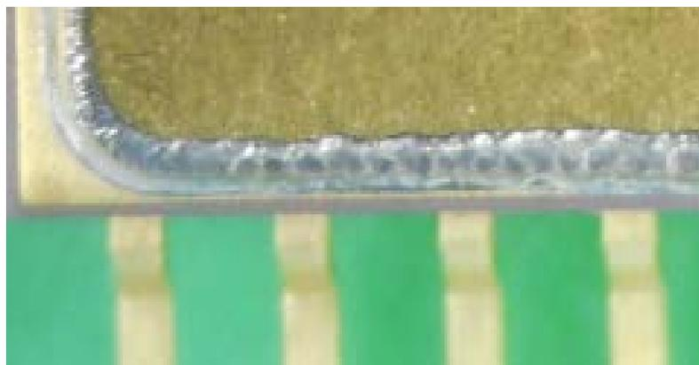
**Figure 11: Seam Sealing using a solder preform.**
