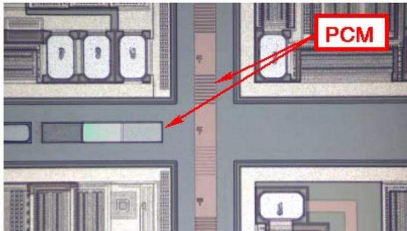
**Figure 1.1: Typical PCM Location before saw**
