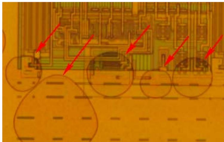
**Figure 9: Die coat blistering cause by nominal sealing temperatures**
