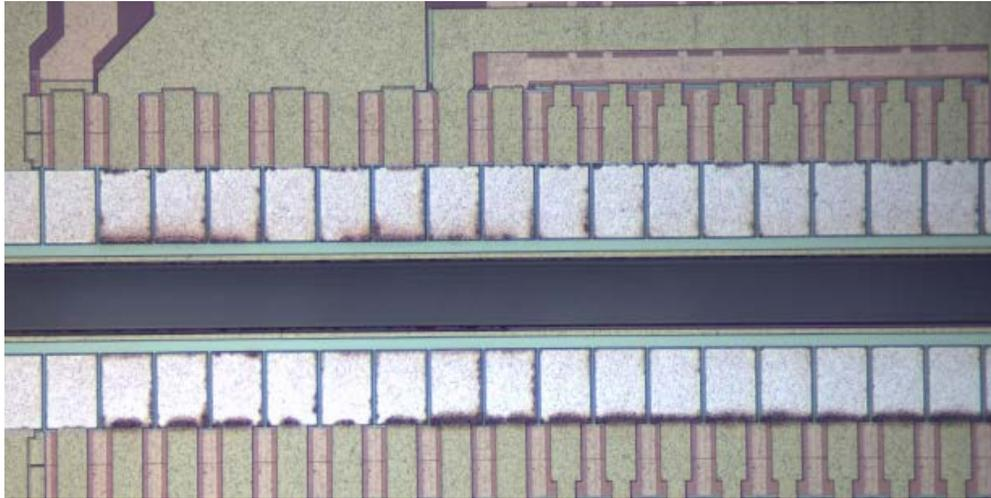
**Figure 1.5: Heavy silicon dust reduced table speed and cut volume**
