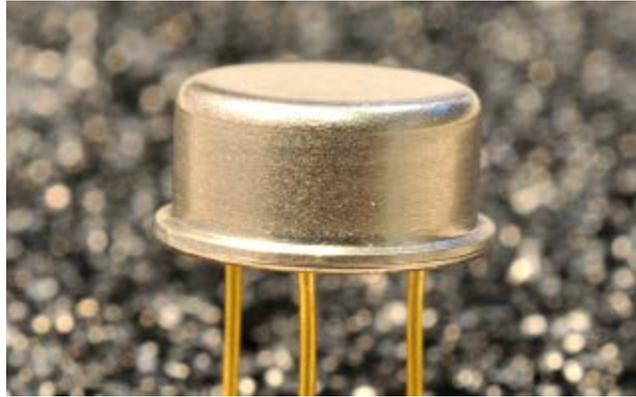
The seam seal process is normally used to create a seal between a metal lid and a metal package body. However, it can also be used to reflow a gold-tin preform between the metal lid and the ceramic package Kovar seal ring. This process also generates heat but it is localized and will not affect the die coat.
