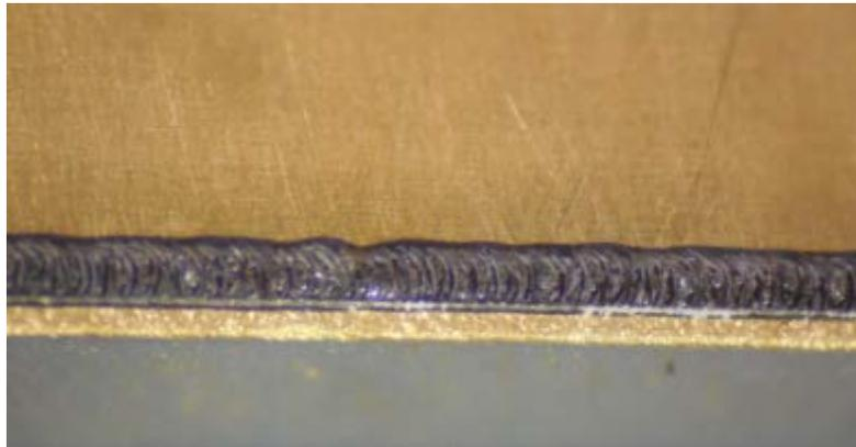
**Figure 10: Standard Seam Sealing.**
