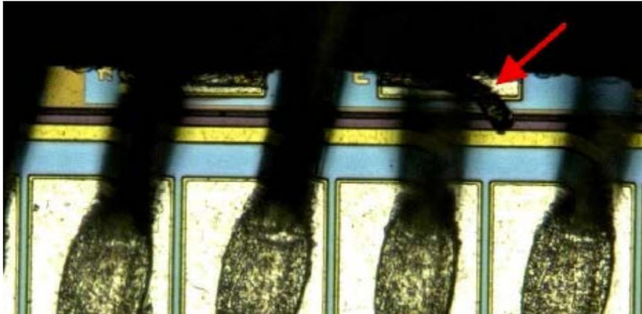
**Figure 1.2: Residual metal from PCM**
