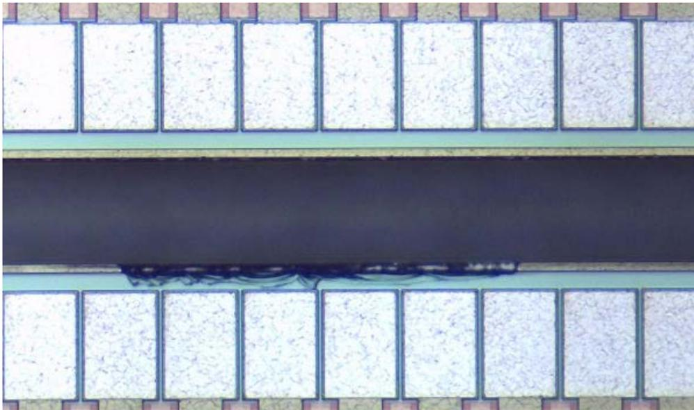
**Figure 1.4: Blade wobble developed using 3030 blade at normal cut speed.**
